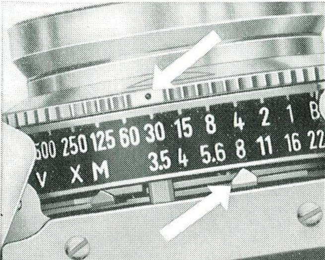
One exposure value will not cover all the aperture and speed settings marked on the shutter, for on turning the speed ring you are eventually bound to reach the limit of either the aperture scale or the speed scale.
