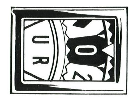
The shaft of the rewind crank underneath the camera carries a red index line which should rotate every time the film is advanced. If it does not move on depressing the Combi-plunger, the film was probably not loaded correctly. In that case remove the camera back again, and secure the beginning of the film leader as described on page 9.
